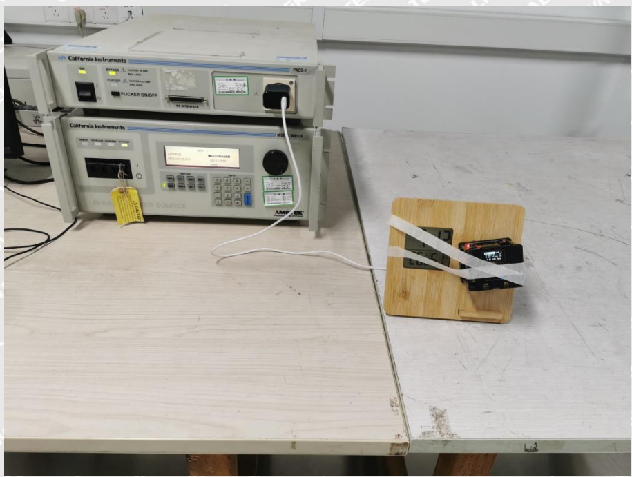
Harmonic/Flicker Test View
